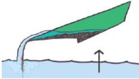
5. Repeat steps 2, 3, and 4, in a vigorous fashion until you have reduced the gravel to an amount which does not go onto the riffles easily, but lays in the bottom front of the Maverick as shown in the drawings
