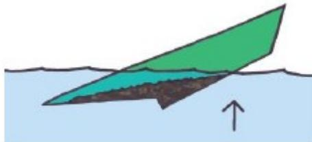
4. Now bring the Maverick straight up making the water flow out like a water fall.\* This action will wash away some of the lighter gravel on the surface while the heavier material gets caught in the riffles. Now dip and repeat this move several times.
