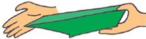
7. Now raise the front of the Maverick up slow enough to let the water drain back off the concentrates without dislodging the gravel and go to the back of the pan.
