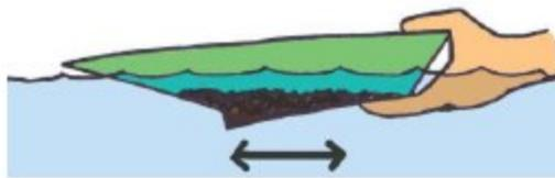
3. Now dip the front of the Maverick into the water to about 2/3rds of the way down at a 45- degree angle. A portion of the gravel will now fall down the riffles.
